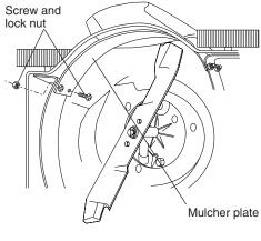
MULCHER PLUG BUILT INTO REAR DOOR
